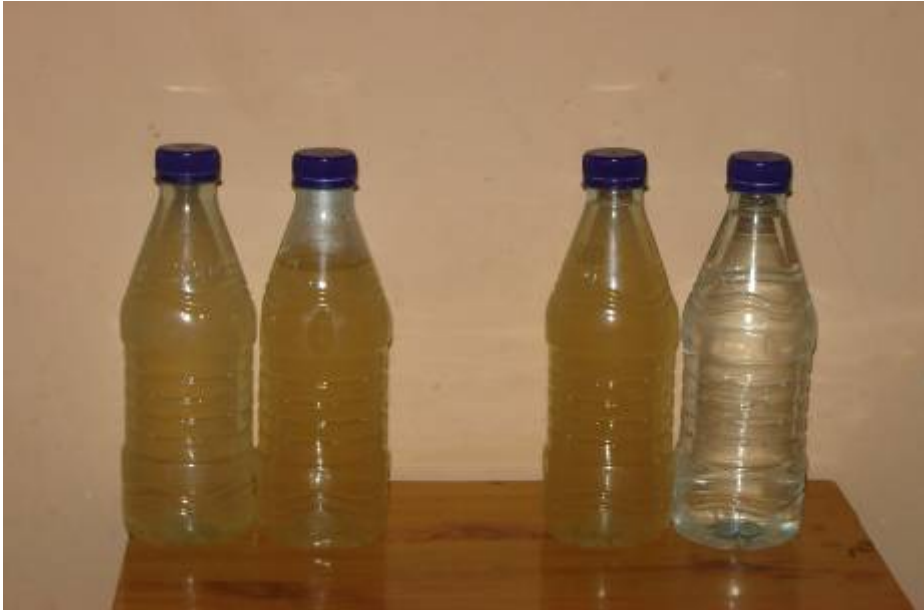
Figure 10. Samples of water taken from Abu Jeyli slow sand filtration system and Sinnar town water supply. From left to right: 1. supernatant water, 2. filtered water from Abu Jeyli, 3. Tap water from Sinnar town water supply. 4. Water sample taken after filtration of water from Sinnar town water supply system and re-filtered using traditional pot container (“Zir”)
