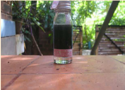
Picture (3.2) H 2 S strip test bottle
