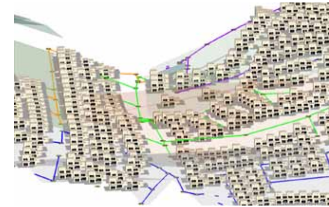
Cluster 3D-Model of collection systems for decentralized wastewater treatment solutions in a sub-urban area of Al-Salt, Jordan
